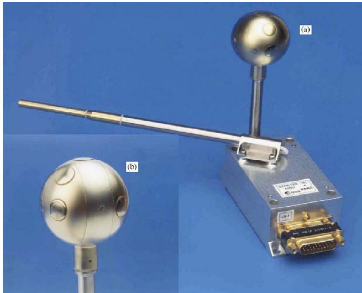
Fig. 2. Overview of the DEMETER Langmuir Probe instrument which is comprised of two Langmuir probe sensors: a cylindrical sensor (diameter 0.6 cm, length 5 cm) and a segmented spherical sensor (sphere diameter 4 cm).
