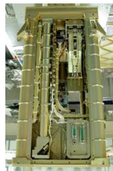
SolACES instrument with subunits (size: 25 x 29 x 60 cm 3 )
