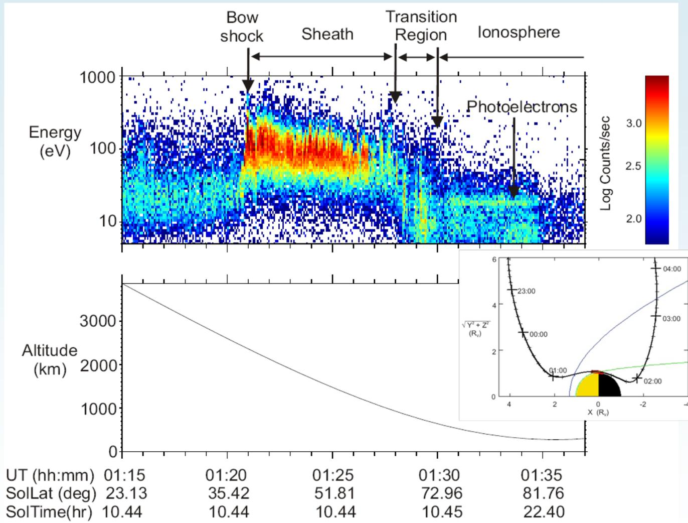
Photoelectron peak energy is not measured at expected value; makes sense if the potential is treated as being negative. Infer high ionospheric electron fluxes.
