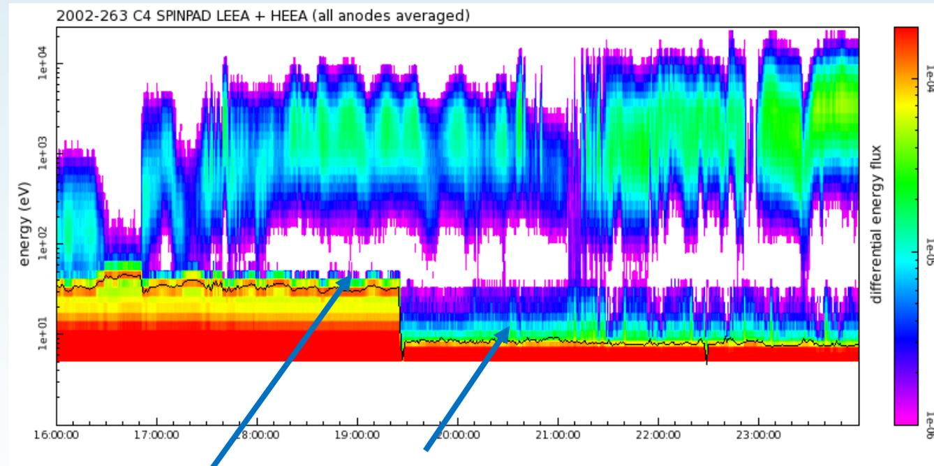
PEACE can only measure cold electrons with good energy resolution when ASPOC is on
