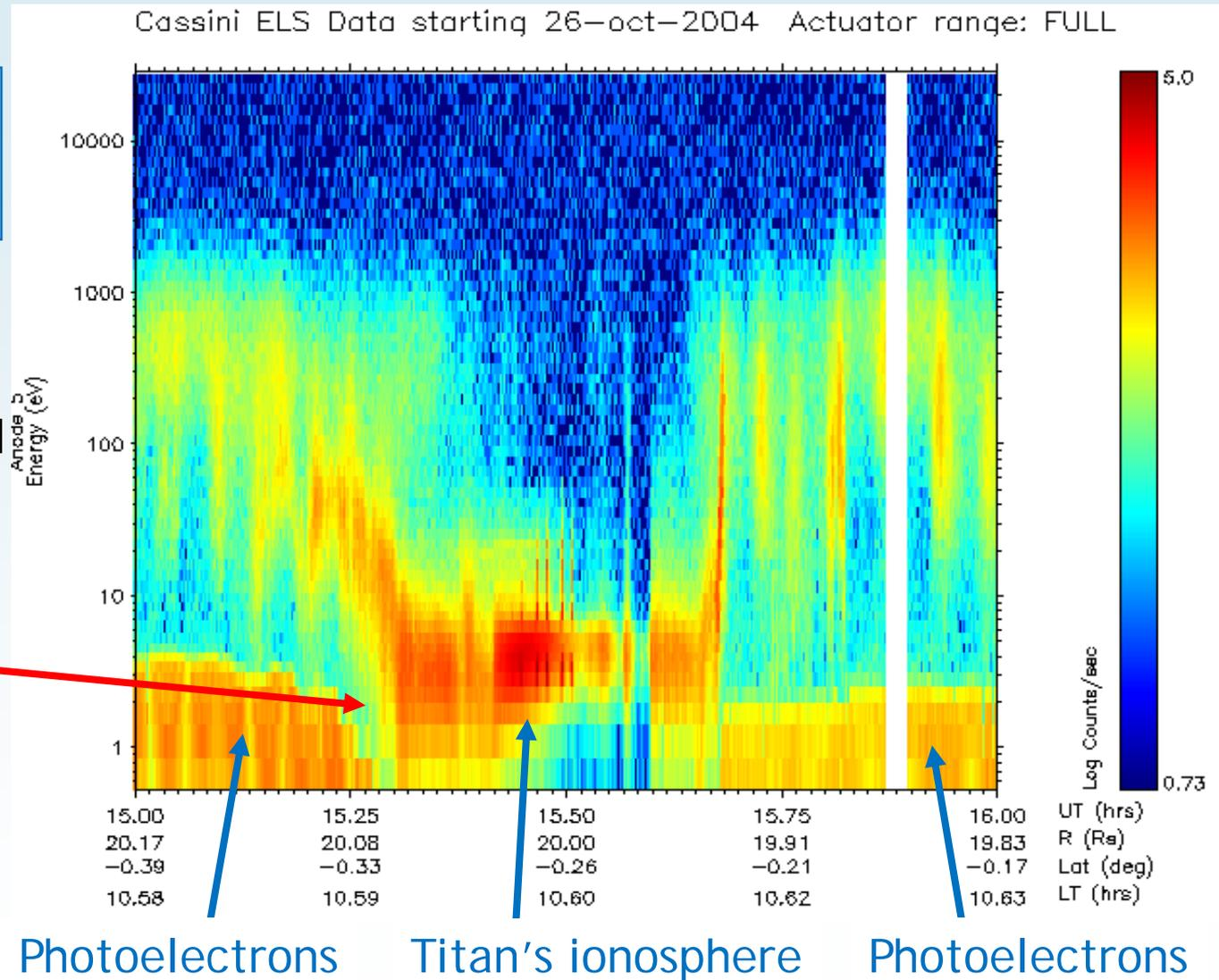
Density comparisons with plasma wave instrument only agree if the potential is treated as being negative
