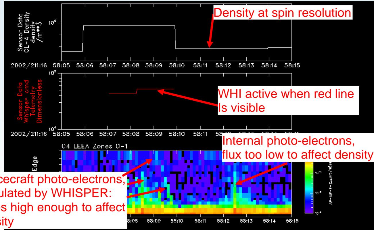
Rapid fluctuations in the current balance during WHI active operations drive photoelectrons to higher energies than  $V_{sc}$ , where they contaminate measurements of the unperturbed plasma electrons. Leads to errors in density moments
