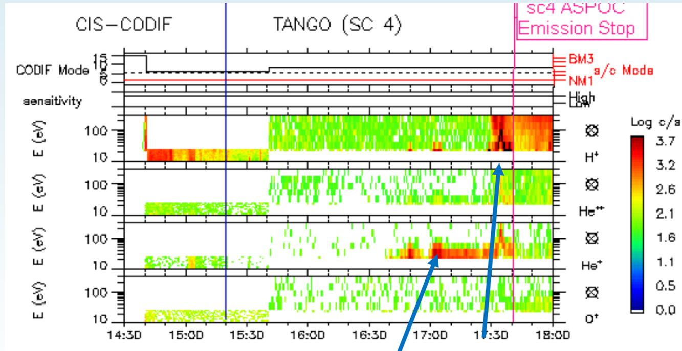
CIS (RPA) can only measure cold electrons with good energy resolution when ASPOC is on
