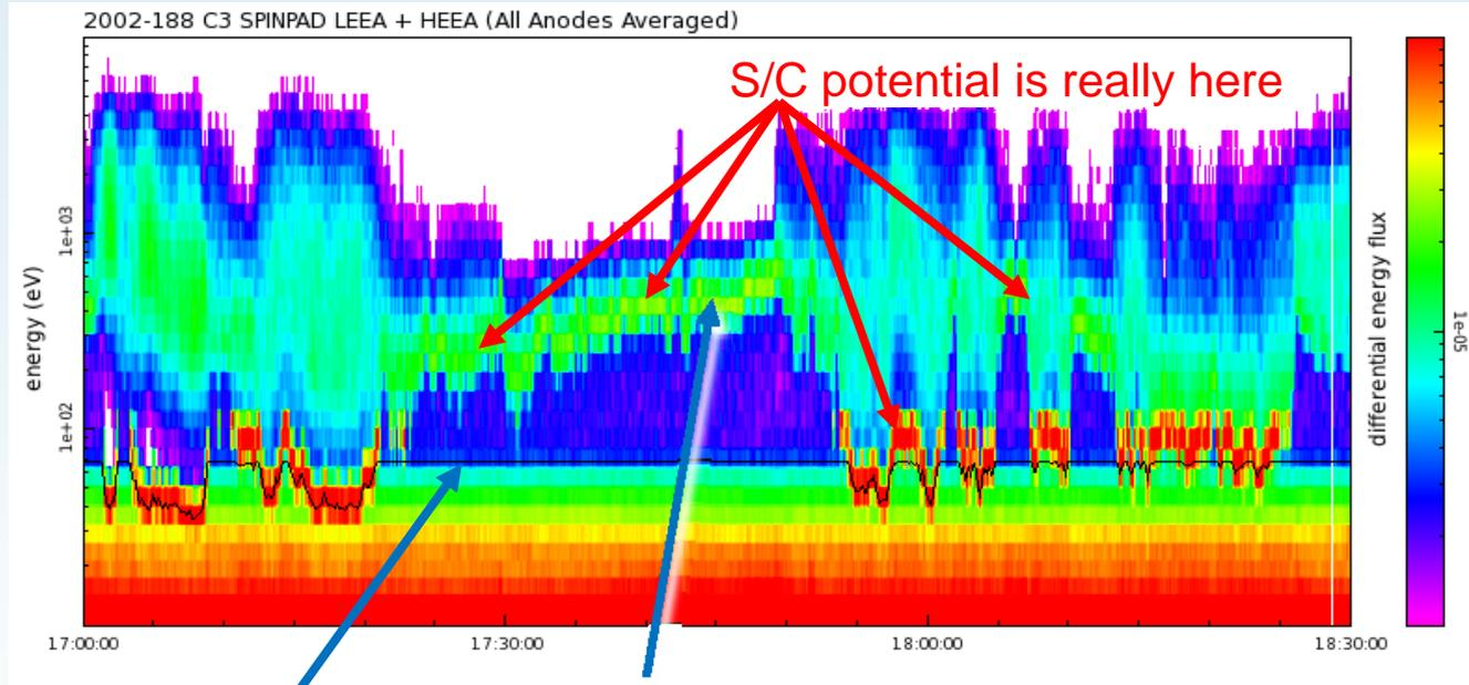
Fluctuations in the current balance drive the spacecraft highly positive in tenuous plasma.
