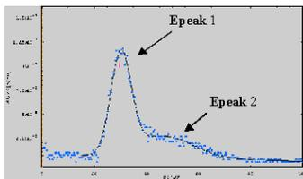
Examples of comparison between PIC simulations of the expected energy spectra and RPA experimental data are reported here below. The simulations, were realized by two different simulation groups: groups from ALTA and groups from ARC and show good agreement. The two groups use two different simulation codes able to simulate charge exchange processes. These work have been performed under the framework of various plasma group meetings held in ESTEC-ESA
