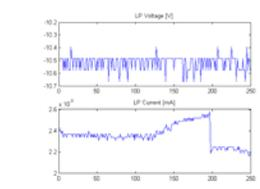
Transient monitoring: Power On and OFF by LP ion / electron current at fixed voltage
