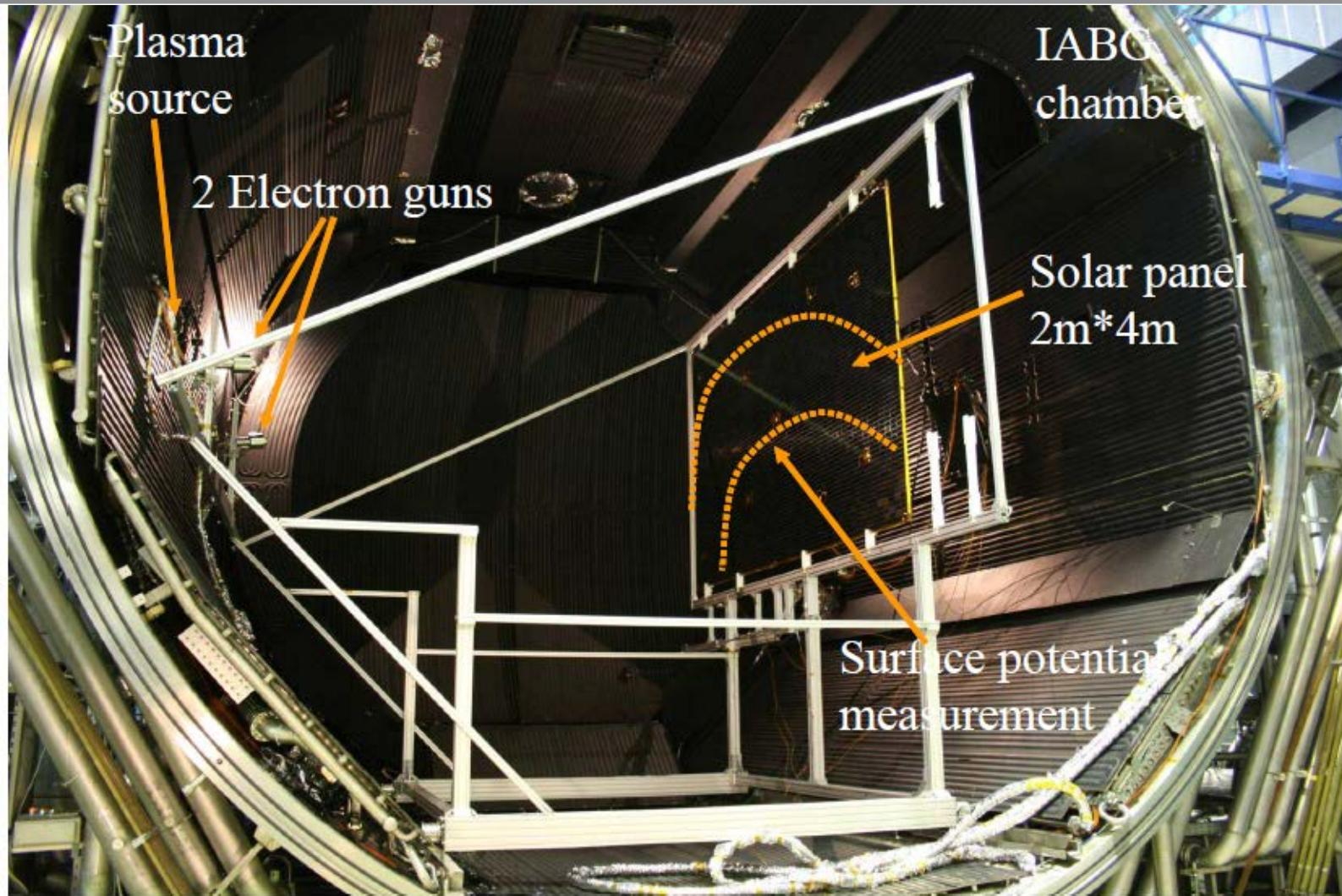
1. IPG (inverted potential gradient) with electron gun
