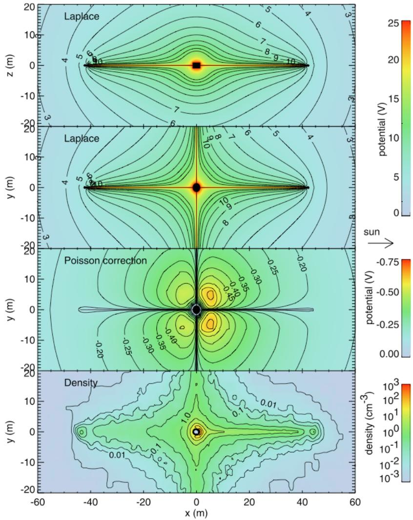
Figure 1 - Simulations of potential and photoelectron density around a Cluster satellite, including fully resolved wire booms. [Cully2007]
