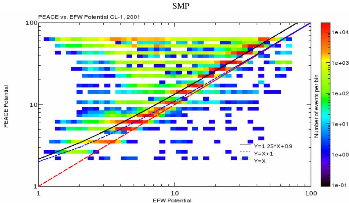
Figure 2 - Cluster satellite potential, as inferred from the PEACE electron measurements, versus the probe-to-spacecraft potential from the EFW probes [Mihaljcic2010]. The black curve is the prediction of the simulations by [Cully2007], which are applicable only in the long Debye length regime, approximately corresponding to potentials above 10 V. SPIS simulations have the potential to apply also to lower potentials (shorter Debye lengths), down to the few volts range.
