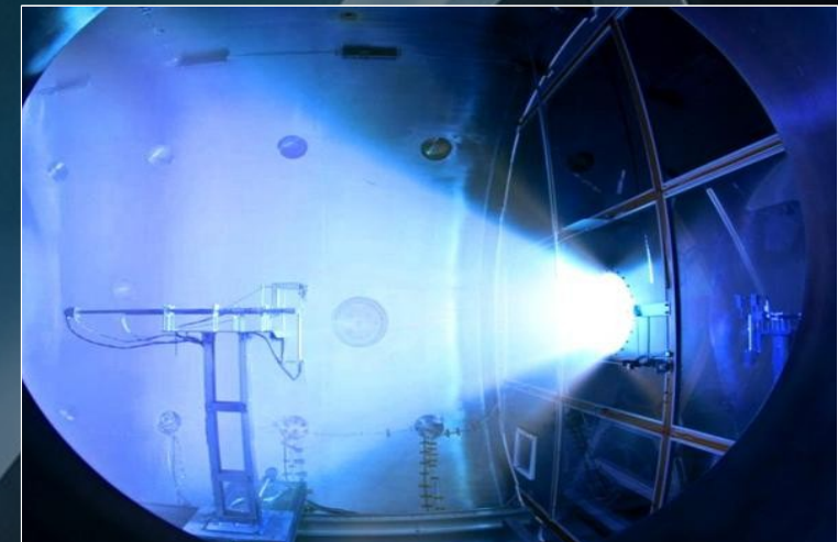
Magnetic Nozzle of VASIMR undergoing test (AARC)
