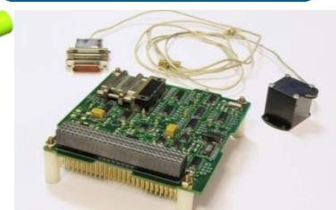
MAGNETOMETER from Imperial College (MAGIC) [ICL, UK]
