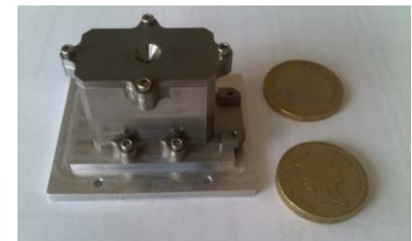
Highly Miniaturised Radiation Monitor (HMRM) [RAL, UK]
