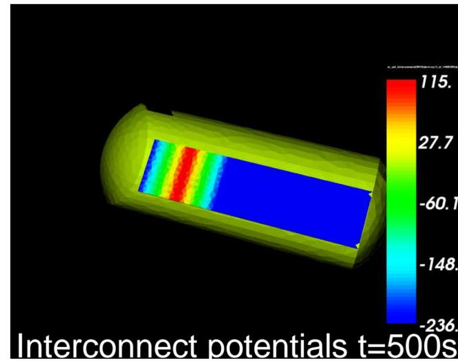
Simulation with  $V_{bus}=350V$ . Initially the interconnects are all positive, But the current they collect changes the whole solar panel potential to  $-240V$
