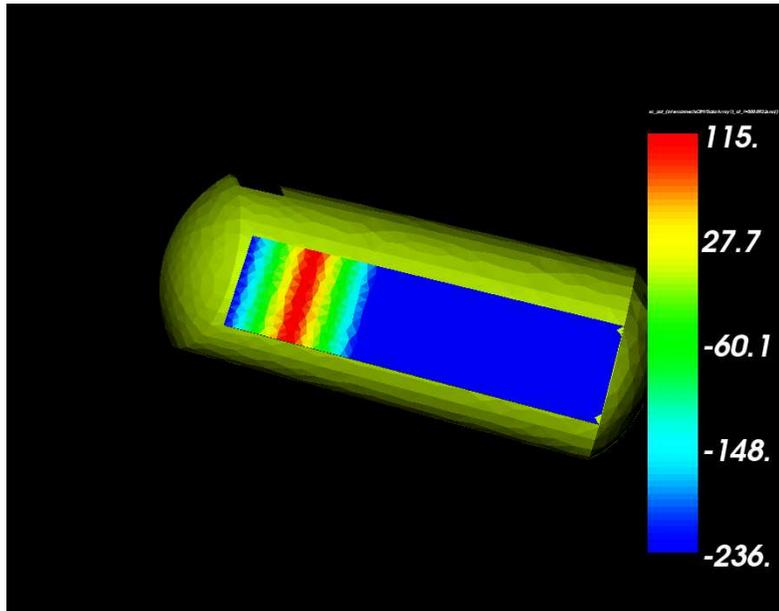
ONERA's JONAS chamber is simulated with the solar panel inside. Environment is tuned to get as close as possible as JONAS one.
