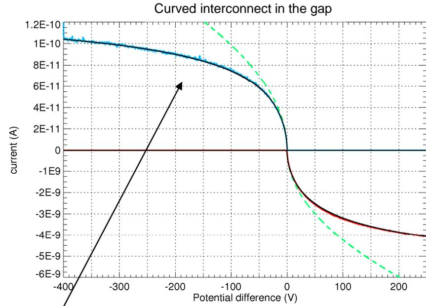
Current saturation due to finite cell surface
