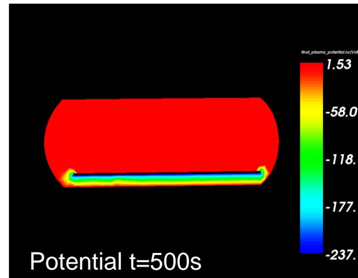
Simulation with  $V_{bus} = 350V$ .
