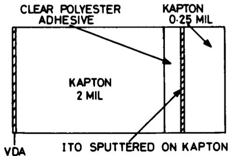
Figure 3. A Further Example of the Improved Version of the Multilayer Thermal Blanket.
