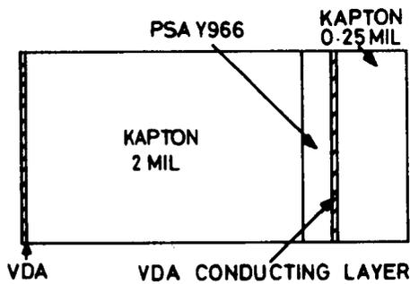
Figure 1. Prototype Version of the Multilayer Thermal Blanket.
