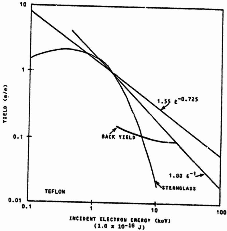
FIGURE 3. BACKSCATTER AND SECONDARY YIELDS FOR NORMALLY INCIDENT ELECTRONS ON TEFLON
