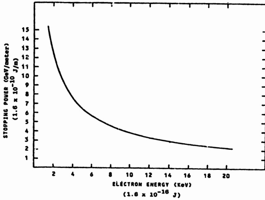
FIGURE 8. ELÉCTRONIC STOPPING POWER OF TEFLON
