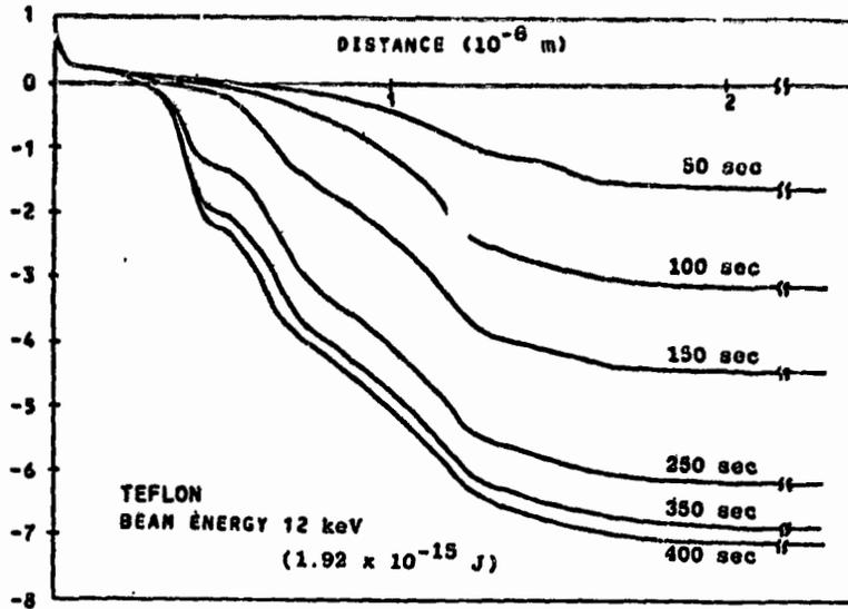
FIGURE 10. TIME HISTORY OF THE ELECTRIC FIELD PROFILE IN TEFLON - NORMALLY INCIDENT 12 keV ELECTRONS
