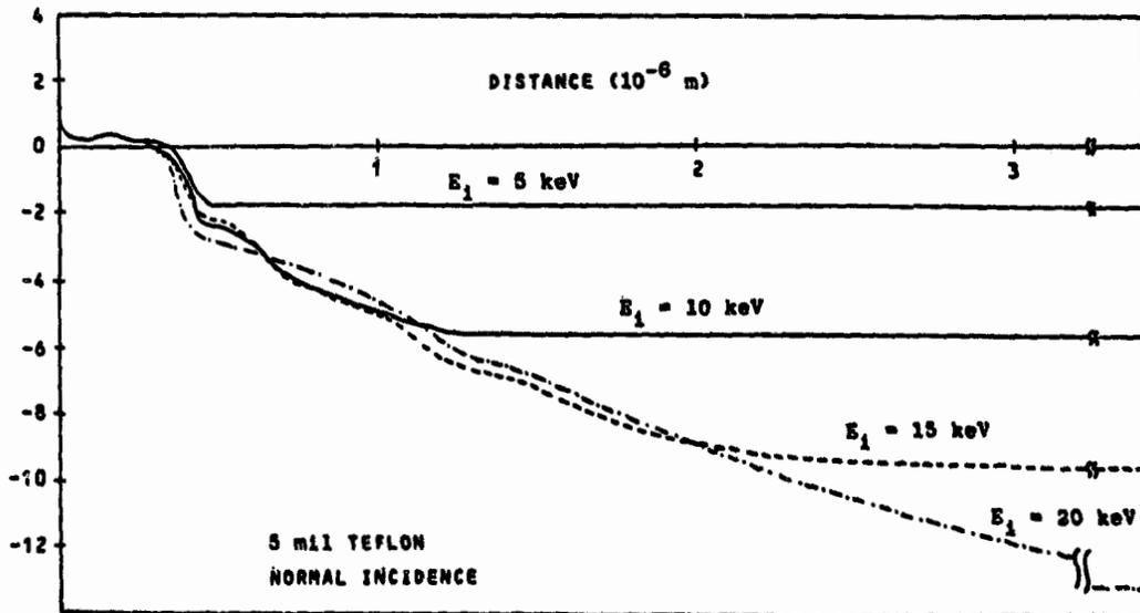
FIGURE 11. SATURATION ELECTRIC FIELD PROFILES IN 5 mil ( $1.27 \times 10^{-4}$  m) TEFLON - NORMALLY INCIDENT ELECTRONS
