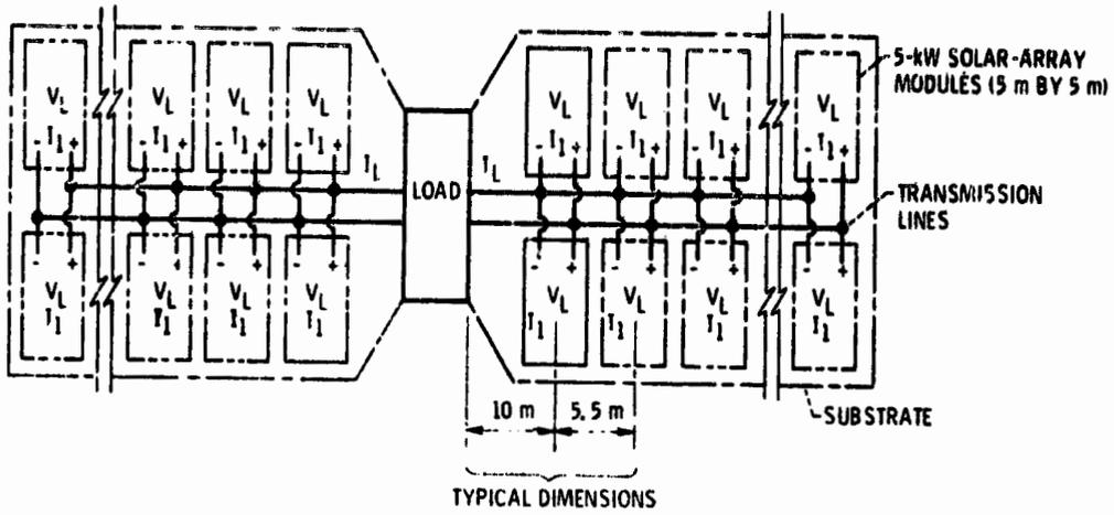
Figure 3. - Conceptual model of large space power system.
