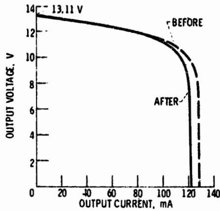
Figure 13. - Degradation in solar-array segment performance after 114-hour test at 4 kilovolts. Solar-array segment area, 100 cm<sup>2</sup>; cell temperature, 49<sup>o</sup> C; light intensity, 1.35, 3 mW/cm<sup>2</sup>. (From ref. 28.)
