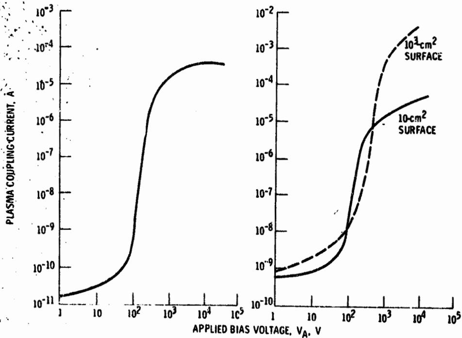
Figure 14. - Current collection phenomenon with pinhole in Kapton film. Plasma density,  $1.7 \times 10^4 \text{ cm}^{-3}$ . Pinhole diameter, 0.038 cm.
