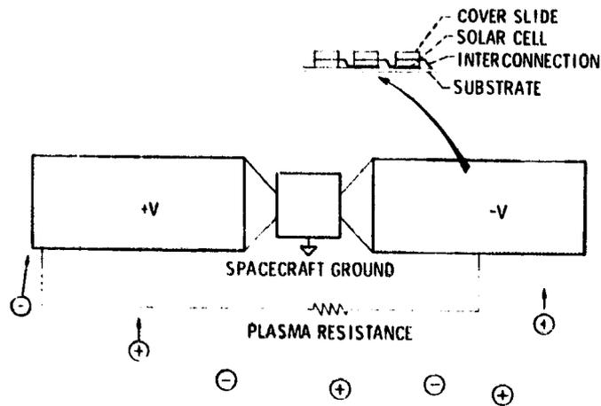
Figure 7. - Spacecraft high-voltage-system - environment interactions.
