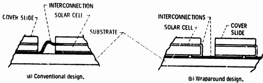
Figure 10. - Solar-array interconnection configurations.
