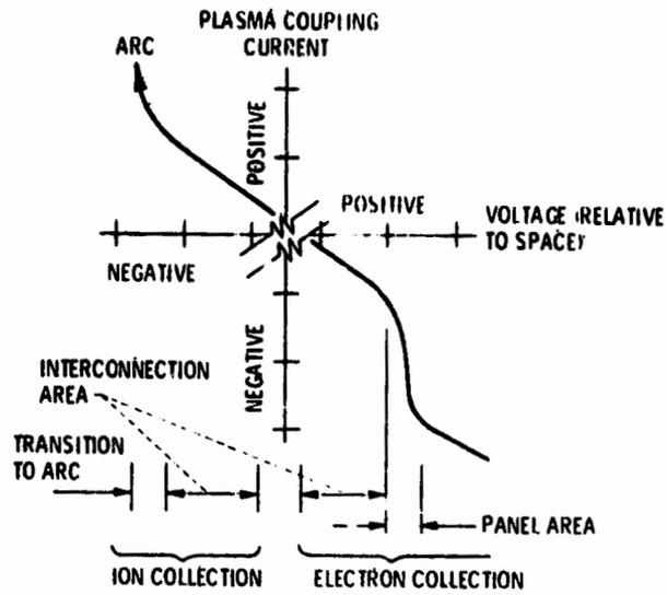
Figure 16. - Solar-array - charged-particle-environment interactions summary.
