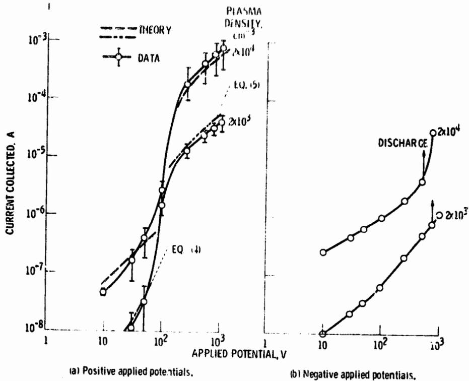
Figure 9. - Plasma coupling currents for solar-array experiment. (From ref. 32.)
