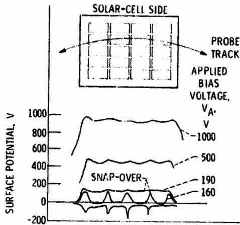
Figure 11. - Surface voltage profiles with wraparound interconnects. (From ref. 12.)
