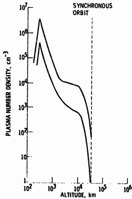
Figure 2. - Plasma number density as function of altitude in equatorial orbit. (From ref. 32.)
