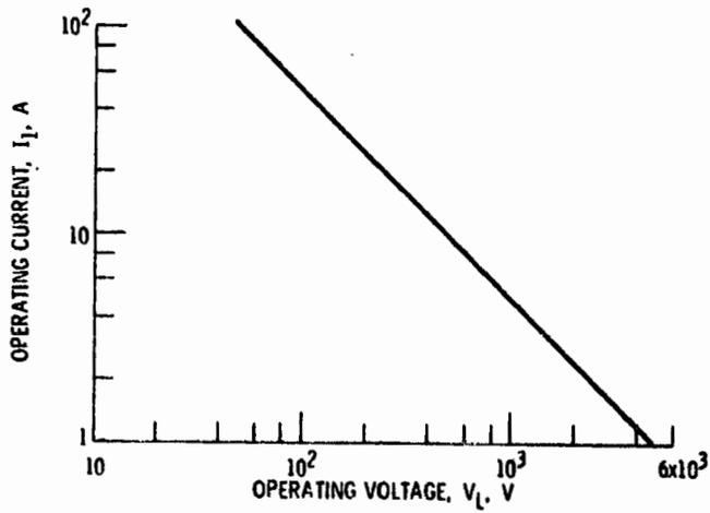
Figure 4. - Load characteristics for 5-kilowatt module.
