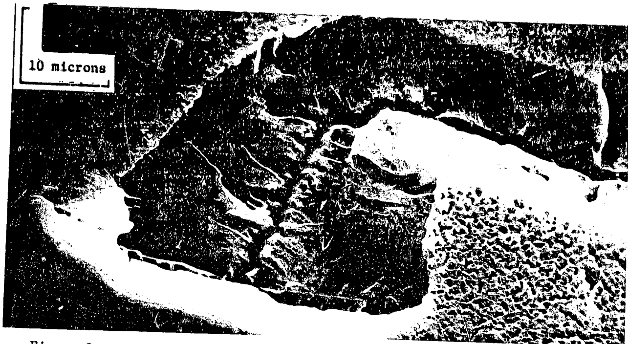
Figure 8. Secondary electron image in a scanning electron microscope of a gold-coated, damaged Mylar specimen.
