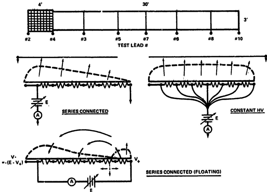
Fig. 4 - Simulated high voltage array electrical configurations (SPL-1; 1977).
