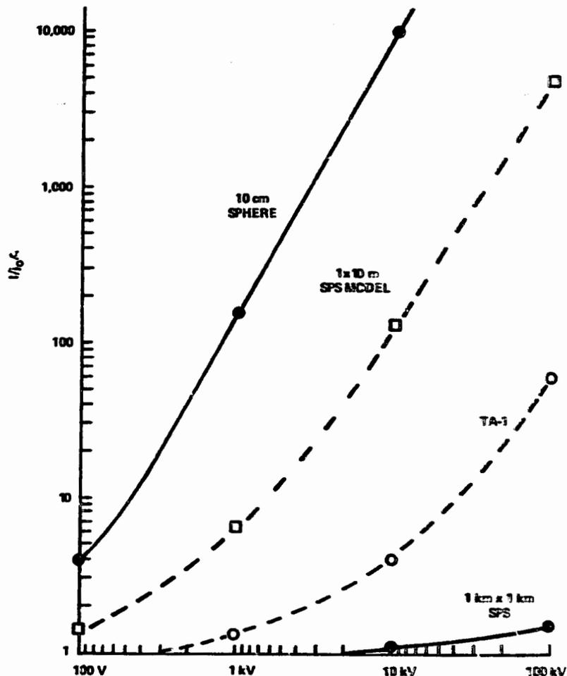
Fig. 2b - Limitation of current multiplication ratio vs voltage expected for collecting objects of increasing size, assuming sheath size limited.
