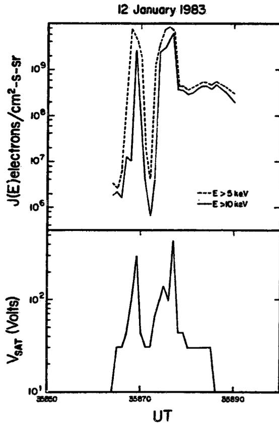
Figure 7. - Integral flux of electrons with energies  $>5$  keV and  $>10$  keV in the poleward inverted-V structure. The bottom panel gives the measured satellite potential as determined from charging peaks in the ion distribution functions at 1-sec intervals.
