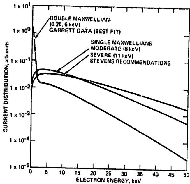
Figure 10. - Electron energy distribution for simulation experiments.
