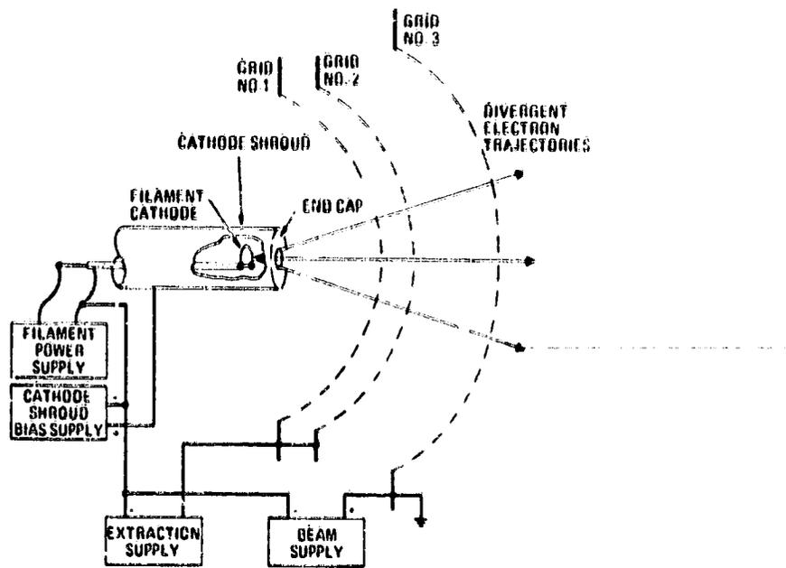
Figure 2. - Electron source (NASA Lewis design).
