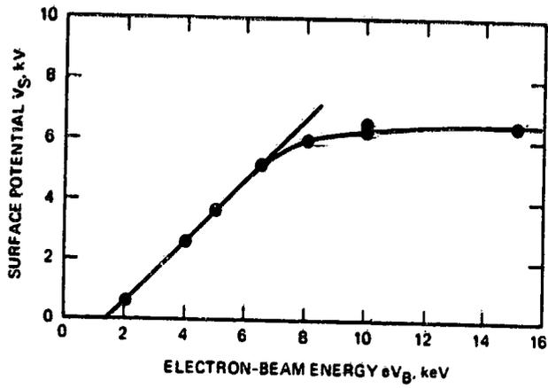
Figure 6. - Surface potential of 25- $\mu\text{m}$ -thick Kapton.
