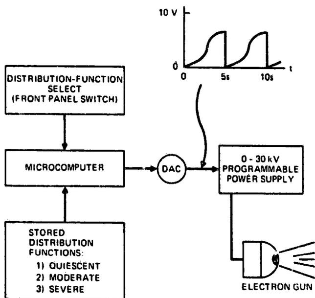
Figure 9. - Block diagram of multienergetic electron beam.
