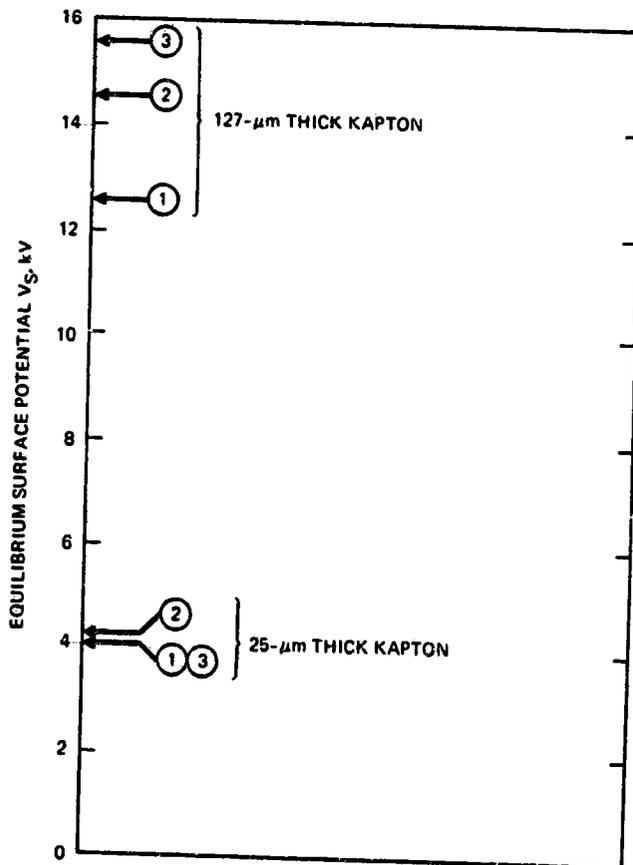
Figure 11. - Equilibrium surface potential of 25- and 127- $\mu\text{m}$ -thick Kapton irradiated by  $3\text{-}\mu\text{Am}^{-2}$  multienergetic electron beam: (1) = "quiescent", (2) = "moderate", (3) = "severe" charging environments.
