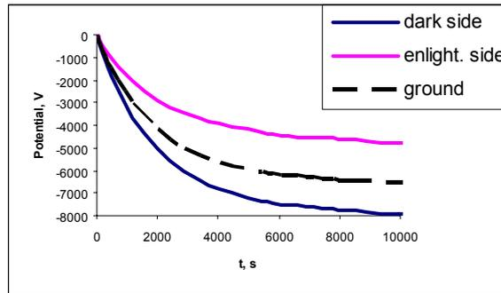
**Figure 5. Potential on various spacecraft surface elements as function of charging time**
