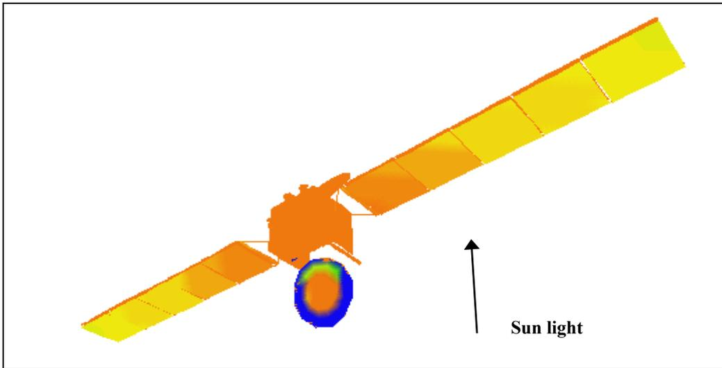
Figure 4. Spacecraft charging at  $t=2.0 \cdot 10^4$  s (steady state)
