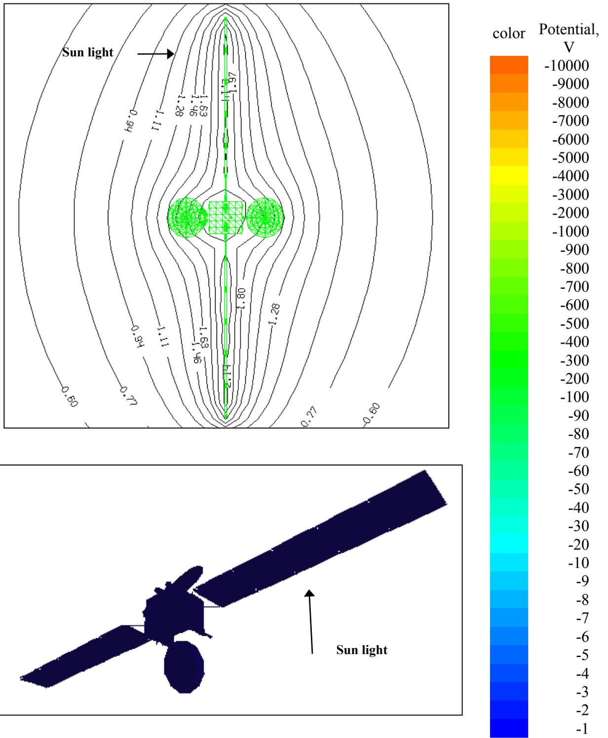
Figure 1. Spacecraft charging at  $t=1.3 \cdot 10^{-3}$  s. Color code scale is on the right
