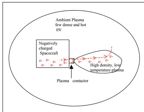
**Figure 3. Plasma contactor principle**
