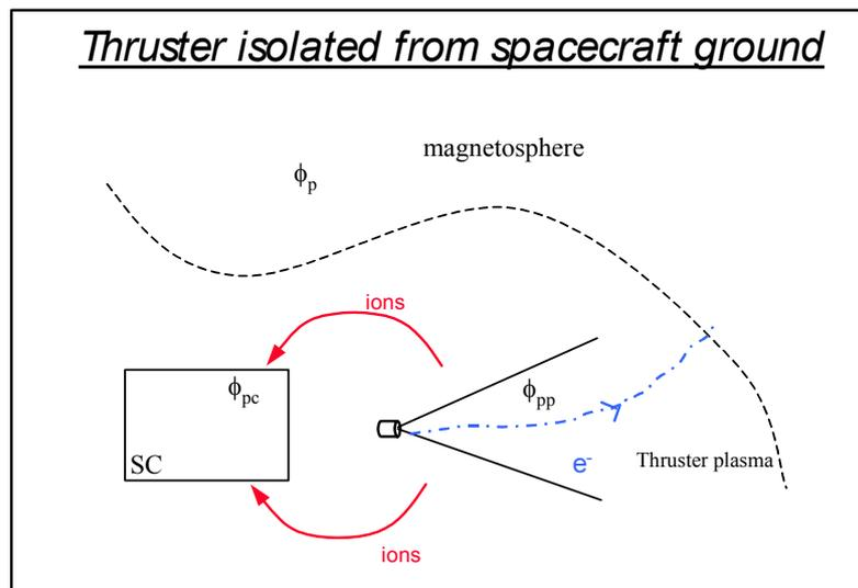
**Figure 12. Thruster isolated from spacecraft ground**
