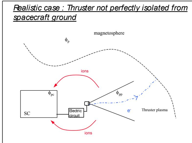
**Figure 13. Thruster not perfectly isolated from spacecraft ground**
