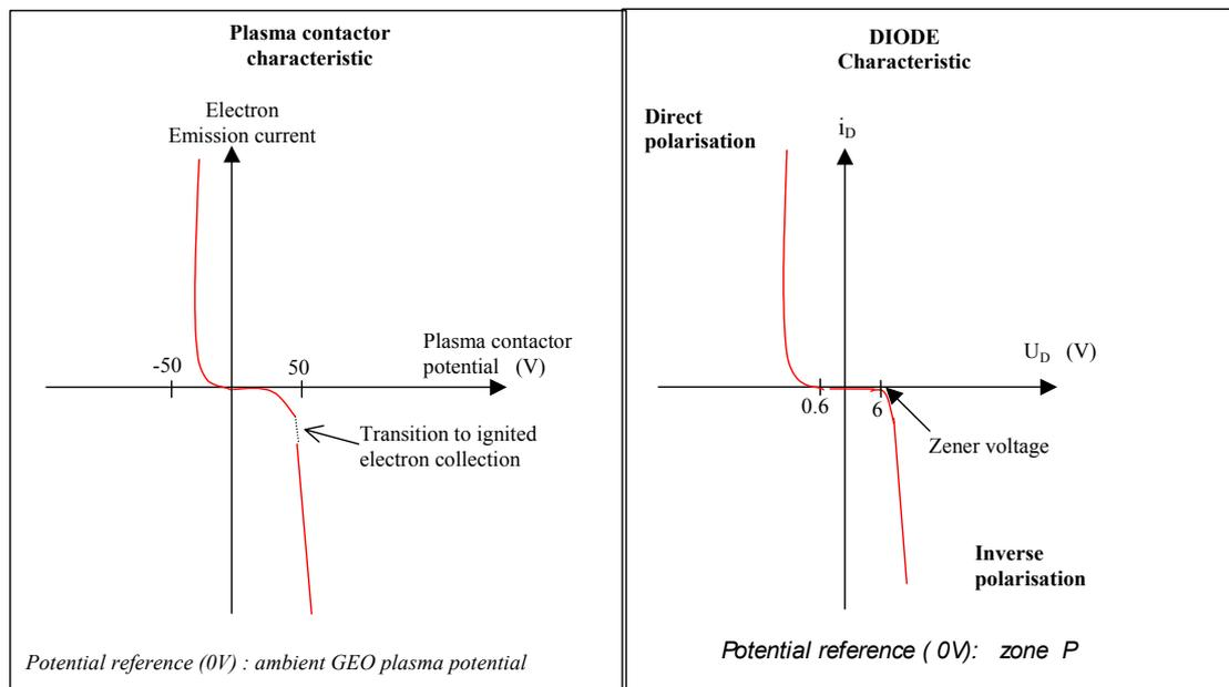
**Figure 9. Diode and plasma contactor current/voltage characteristic**
