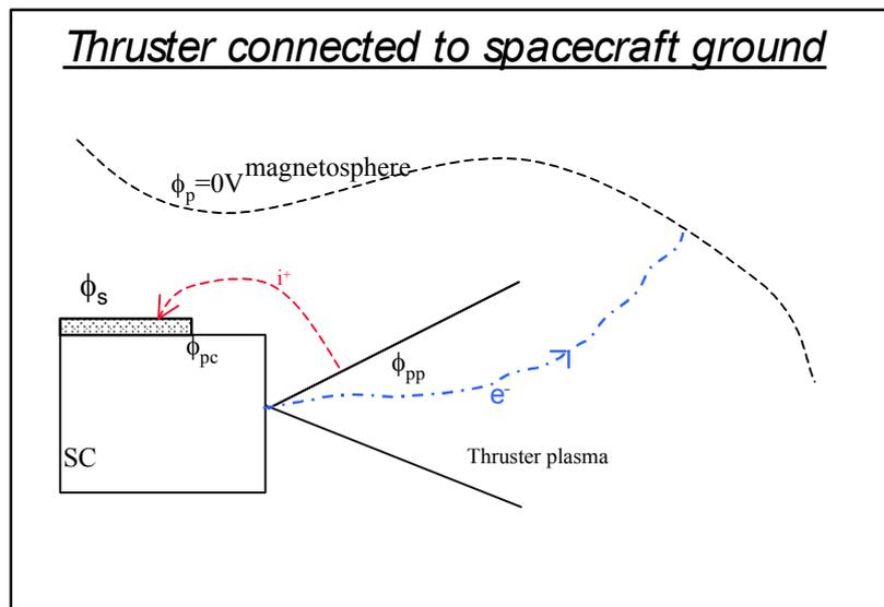
**Figure 11. Thruster connected to spacecraft ground**
