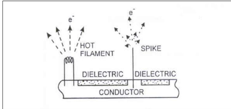
**Figure 1. Electron emissions from a sharp spike and a hot filament**
