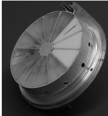
Figure 1. Motor-driven monitor: dielectric samples and embedded probes in the motor-driven monitor.
