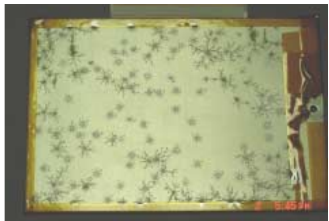
Figure 3. Post-Test Sample with Arcing Damage
