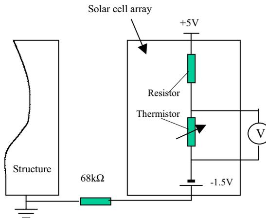
Figure 2. Circuit diagram of electrical ground floating experiment
