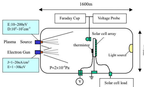
Figure 1. Configuration of solar array charging experiment
