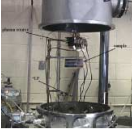
Fig.1. Small vacuum chamber is shown with sample installed
