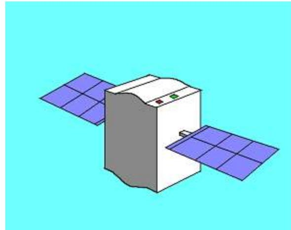
**Figure 2.** A schematic diagram of the DSCS satellite. The small kapton and quartz surfaces and the ion flux detector (not shown) are on the ram side of the satellite.
