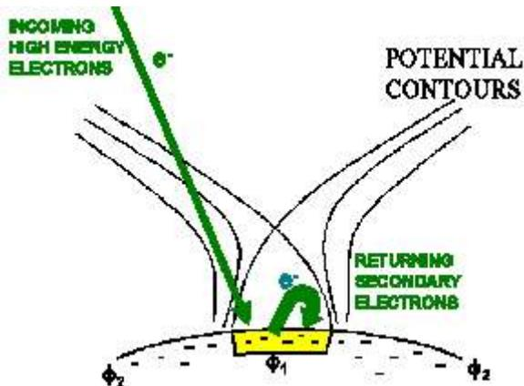
**Figure 1.** A potential well with a saddle point above a small surface surrounded by a large surface, which is at a higher level negative potential relative to the well. The secondary electrons from the small surface are trapped in the well.
