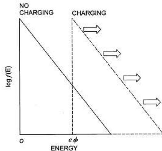
**Figure 3.** Shift of the Maxwellian distribution function of the repelled charge species. The magnitude of the shift indicates the charging level.
