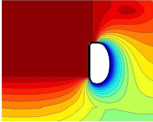
Figure 3. Potential map in the analyser plane [ $V_s = +4$  V;  $V_h = -4$  V; potential step: 0.2 V]
