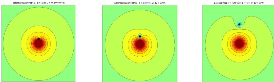
Figure 6. Potential between two conductive spheres for various distances (sphere radius: R and r for the satellite and the detector respectively; d: distance between centers; V and v: satellite and detector potentials; dV: contour step).
