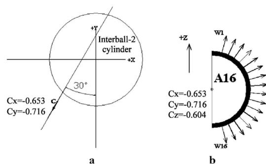
Figure 2. HYPERBOLOID ion analyser A16 (a: location of the analyser plane; b: directions of the windows)
