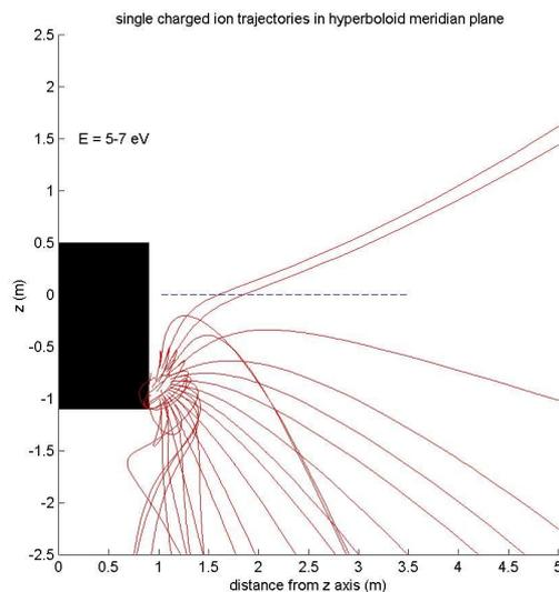
Figure 4. Projection of 3D ion trajectories on the A16 analyser plane for  $V_s = 12$  V and  $V_h = 4$  V (see text).
