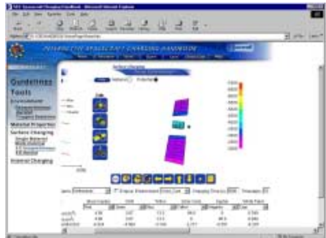
Figure 8. SEE Interactive Charging Handbook charging results. Shown are the potentials on the sunlit side of the solar arrays and spacecraft body. The largest potential is -3 kV.
