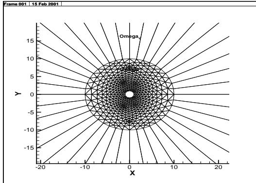
Due to the thickness of dielectric, the array resulting of this Galerkin resolution must be preconditioned. While the thruster is OFF, the space charge is neglected, but when it is ON, we have to fix potential inside the SPT-thrust, and to take care about space charge coming from the boundary of the thrust.
