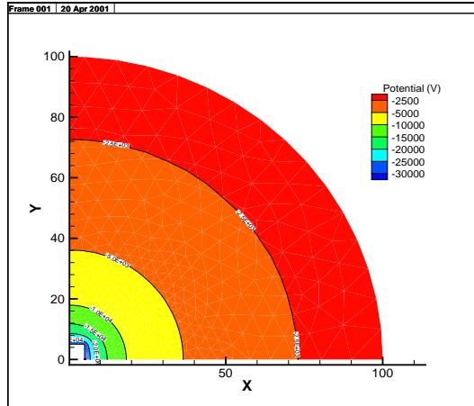
On some cells exposed from the secondary plasma ions, the calculated current coming from slow ions is about  $2A/m^2$ . With this current the potential go quickly to zero when the thruster is switch ON. But another equilibrium is not reached since we have not included currents from thruster electrons. Also, these results have not yet validated.
