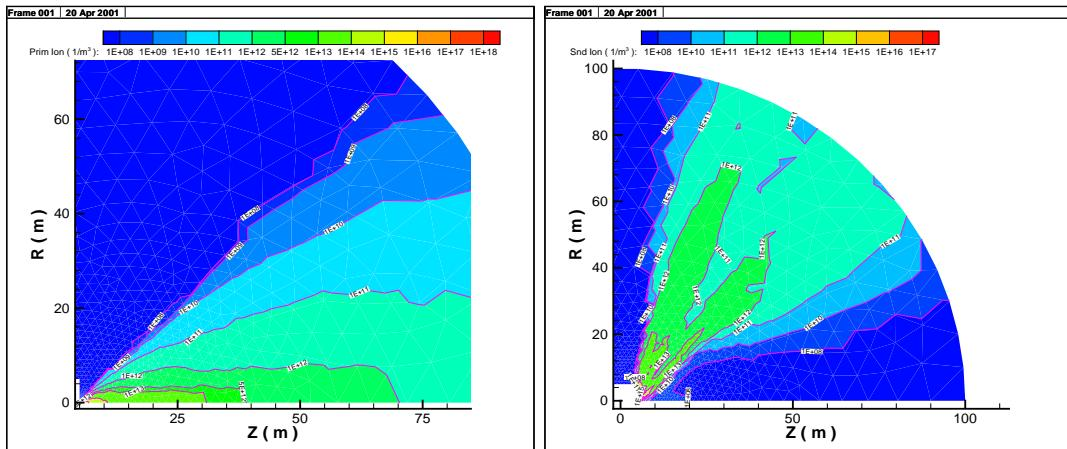
Because the neutrality is imposed inside the center of the plume, the isopotential are the same that isodensity. We can notice on the primary ions density, that electric field push slow ions on the boundary of the plume and some of them impinge satellite surfaces. This is in good agreement with Samanta Roy results on backflow contamination. [9]
