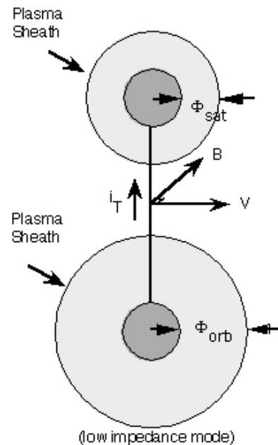
**Figure 4. Schematic of an electrodynamic tether system flowing current.**
