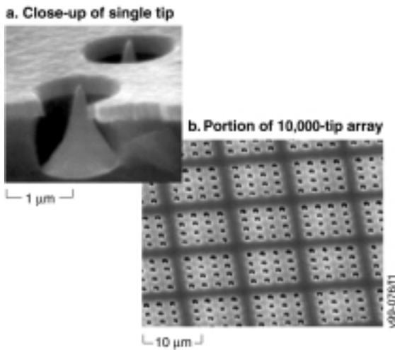
**Figure 1. (a) Electron micrograph close-up of Spindt cathode tips, and (b) close-up of a section of a cathode array.**
