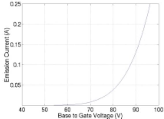
**Figure 3. Modeled values of emitted current vs. gate voltage for 5-million-tip Spindt cathode array.**
