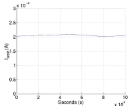
**Figure 5. Plot of emitted current over time with a Spindt cathode under feedback control.**
