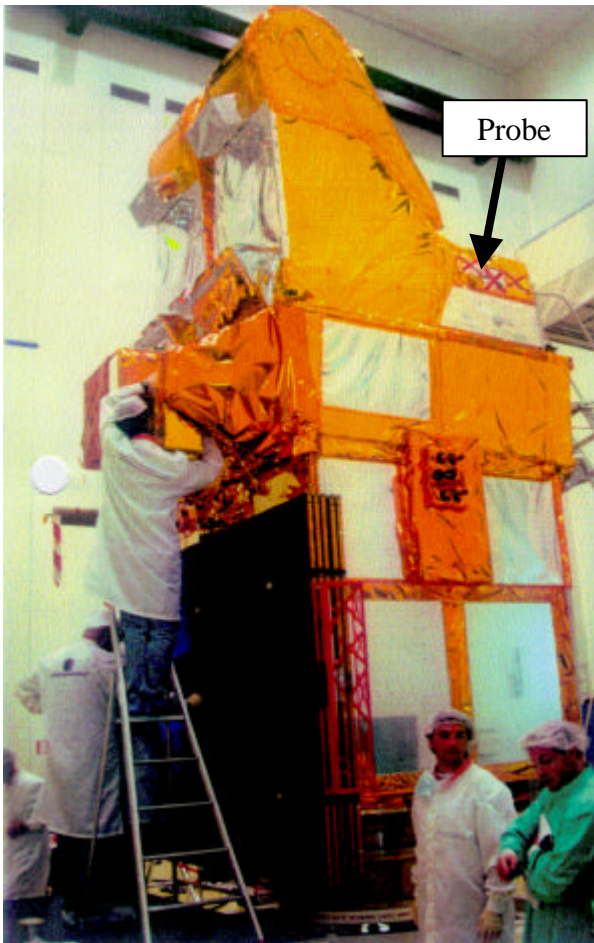
Figure 3- Voltage probe on the wake side
