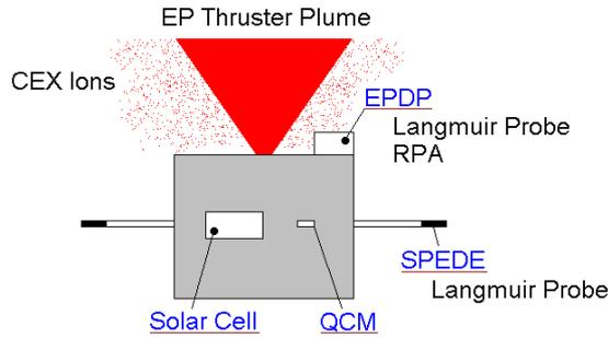
**Figure 1 Schematic Instrument Location on SMART-1**
