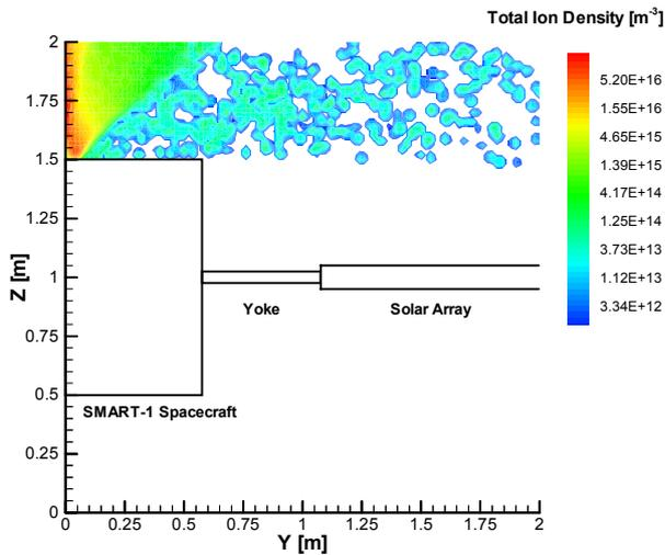
**Figure 7** y-z Plot of Ion Density through middle of SMART-1
