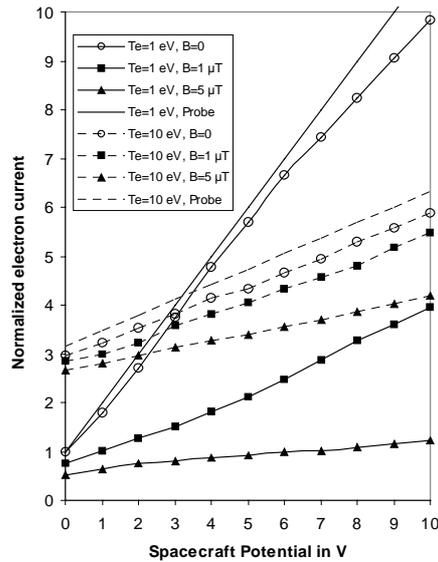
Figure 4. Current-voltage characteristics of collected plasma electrons for different values of  $B_0$ . All currents are normalized with respect to the thermal current.
