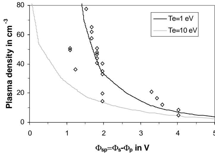
Figure 6. Results of diagnostic measurements: the diamonds show the measurements of  $N_e$  and  $\Phi_{sp}$ . The  $N_e(\Phi_{sp})$  curve was deduced from the  $N_e(\Phi_s)$  relation for  $B_0=1 \mu T$  by estimating analytically the probe potential  $\Phi_p$  with respect to the plasma.
