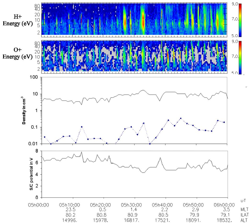
Figure 7. From top to bottom : Ion energy-time spectrograms of H<sup>+</sup> and O<sup>+</sup> ions recorded by the Hyperboloid experiment, calculations of the plasma density from numerical relations (solid) and from ion measurements (dot), and measurements of the S/C potential versus time.
