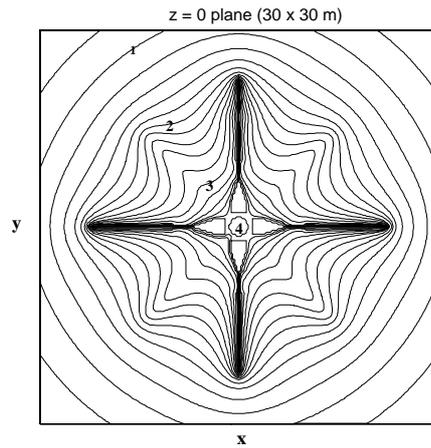
Figure 2. Equipotential contours of the potential distribution in the solar panel plane x-y. The S/C body is at + 4V.
