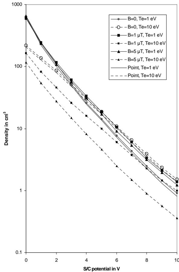
Figure 5. The plasma density as a function of the floating S/C potential for different values of  $T_e$  and  $B_0$ , as summarized in Table 1.
