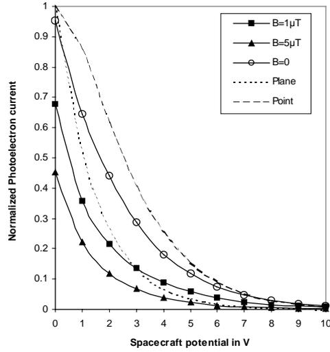
Figure 3. Current-voltage characteristics of ejected photoelectrons for different values of  $B_0$ . All currents are normalized with respect to the photoelectron saturation current.
