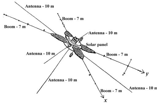
Figure 1. Geometric structure of Interball AP.
