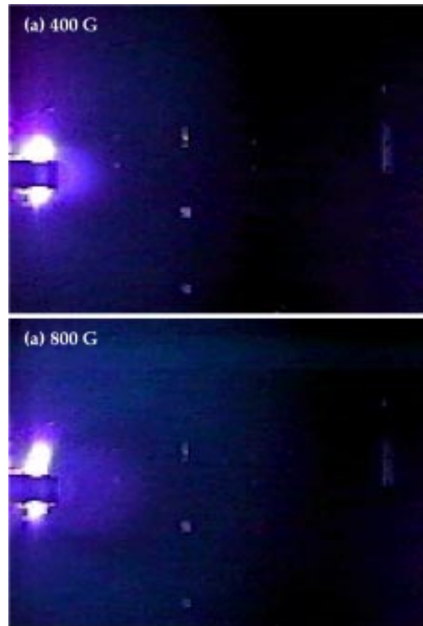
Figure 5. Interaction of an artificial magnetosphere and a surrogate solar wind showing the presence of a magnetopause (dark slightly curved vertical region) separating the opposing plasmas. Note the translation of the magnetopause location from (a) \sim 0.55 the width of the image to (b) \sim 0.75 the width.
