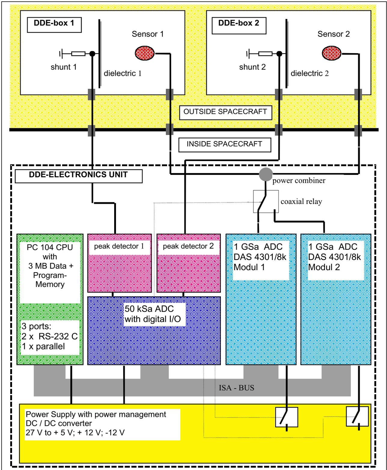
**Figure 3:** Discharge Detector Experiment functional block diagram
