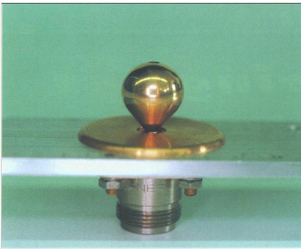
**Figure 2: Electric field probe (D-dot antenna)**
