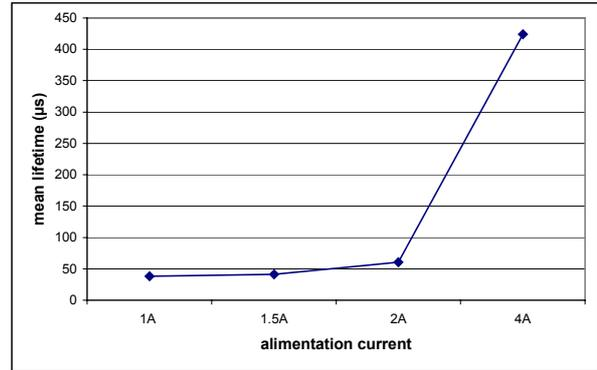
**Figure 7:** lifetime as a current function (zinc sample). Applied voltage=40V
