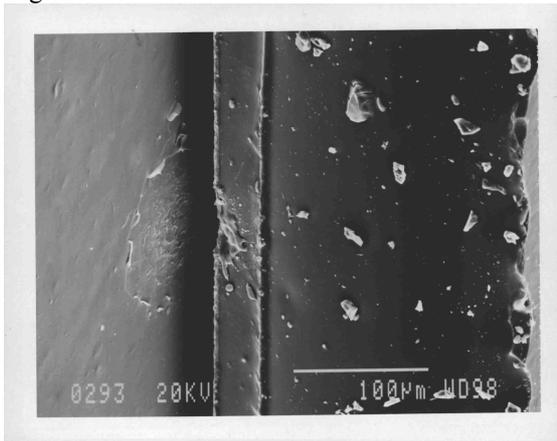
**Figure 4:** SEM recording of a solar cell sample (left part: kapton, middle: silver interconnect, left part: cell and cover-glass)
