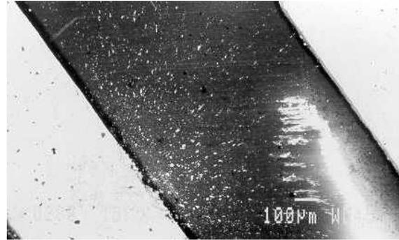
**Figure 5:** SEM recording of a zinc sample (dark layer in the centre : epoxy insulator, white layers on both sides are the zinc cathode –left- and anode –right). The large white cloud with striations on the bottom right of the epoxy layer is an artefact from charging effects of this surface under the SEM.
