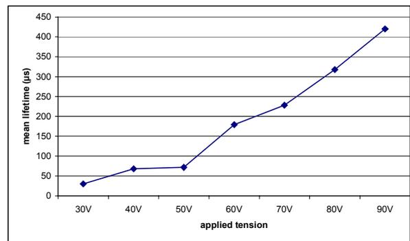
**Figure 8:** lifetime as an applied voltage function (copper sample). Current=4A
