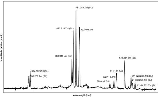
**Figure 3:** spectroscopic data obtained during a secondary discharge on a zinc sample: all the identified lines are zinc lines.
