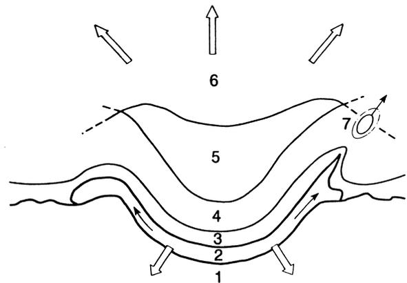
**Figure 1:** spot structure: 1- solid metal cathode below the spot; 2- molten metal layer (0.2-0.5 $\mu\text{m}$ ); 3- space charge layer (0.005-0.01 $\mu\text{m}$ ); 4- ionisation and thermalisation layer (size 0.1-0.5  $\mu\text{m}$ ); 5- dense central spot plasma (5-20  $\mu\text{m}$ ); 6- plasma expansion region; 7- ejection of molten droplets (size: 0.1-100 $\mu\text{m}$ ). Ref: Farral, Lafferty: Vacuum arcs
