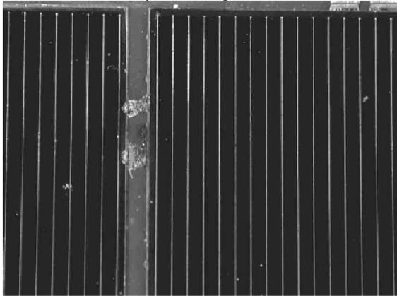
**Figure 6:** photo of a solar cell sample. One can see clearly visible damages (molten metal between the two adjacent cells (scale: gap=1mm).
