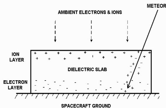
**Figure 4. An ionization channel produced by a meteor impact. The channel may initiate a hazardous discharge in a differentially charged system.**
