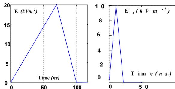
Figure 3: ESD induced E-field waveforms #1 and #2
