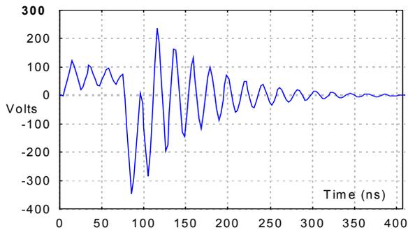
Figure 6 : Time domain Thevenin generator computed with the CRIPTE code at the input level of the DUT (1 V/m hybrid plane wave injection).
