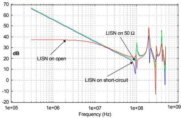
Figure 9: Ratio between the voltage computed on a 50 Ω DUT when a 1 V localised generator is applied in the middle of the wiring and the voltage on the same load for an hybrid plane wave excitation.
