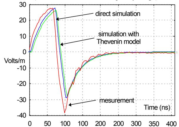
Figure 8: Time domain voltage measured on a 50  $\Omega$  load on the DUT (all loads equal to 50  $\Omega$ )
