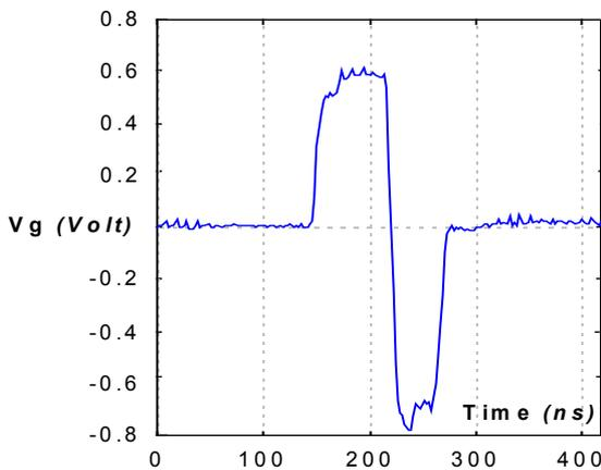
Figure 10: Derivative of waveform 1 generated by the digital/analog converter, amplified and injected with the current injector
