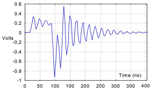
Figure 7 : Time domain Thevenin generator at the output of the digital/analog converter and injected on the experimental set-up at the input level of the DUT (1 V/m hybrid plane wave injection)
