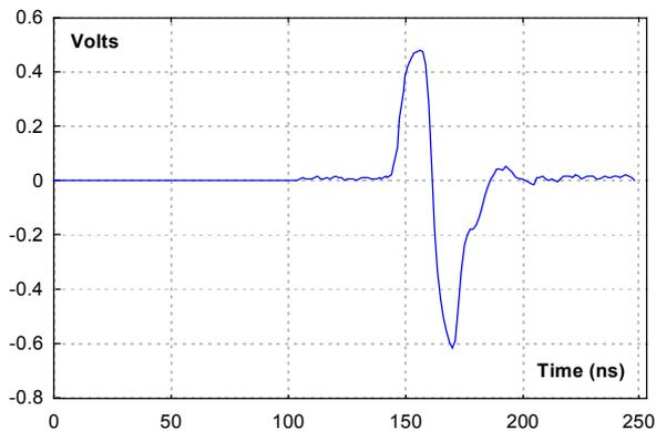
Figure 12: Derivative of waveform 2 generated with the digital/analog converter, amplified and injected with the current injector.
