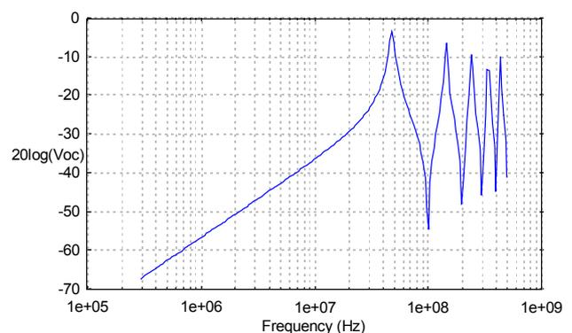
Figure 5 : Thevenin equivalent generator computed with CRIPTE code at the input level of the DUT (1 V/m hybrid plane wave injection).
