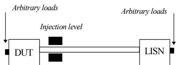
Figure 4 : Schematics of the validation set-up
