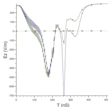
Figure 2: Electric Field pulse at the left edge of the panel (1.5 m from discharge site) which emphasises a narrow peak at the end of the propagation.
