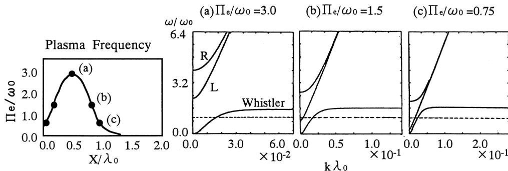
Figure 3.  $\omega-k$  diagram corresponding to each position of the reentry plasma layer. The dashed line in each panel represents the frequency of the radiated wave  $\omega_0$ .
