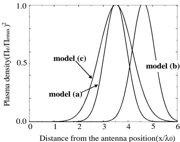
Figure 5. Models of plasma layer used in the computer experiments
