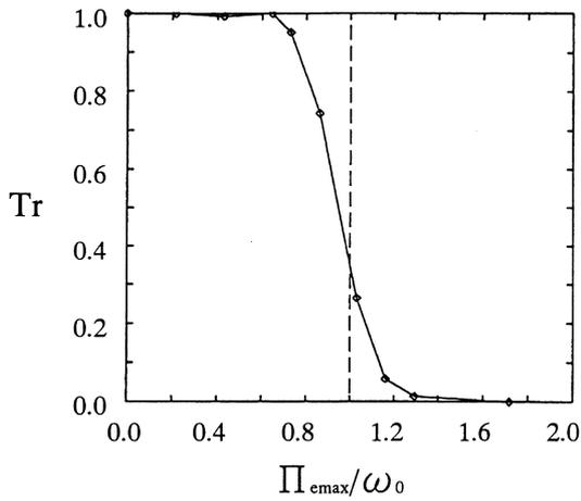
Figure 2. Transmission ratio of radio wave emitted from a reentry vehicle
