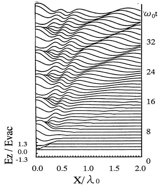
Figure 4. Snapshots of spatial profile of  $E_z$  component at different times superimposed vertically.
