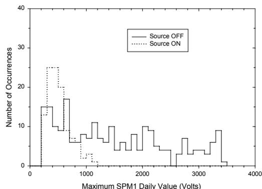
Figure 2. Histograms of maximum daily SPM1 charging levels with the source on and off.
