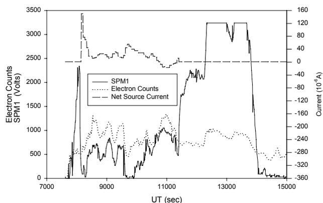
Figure 1. Electron, SPM and Source current data for charging event during day 115 of 1998.
