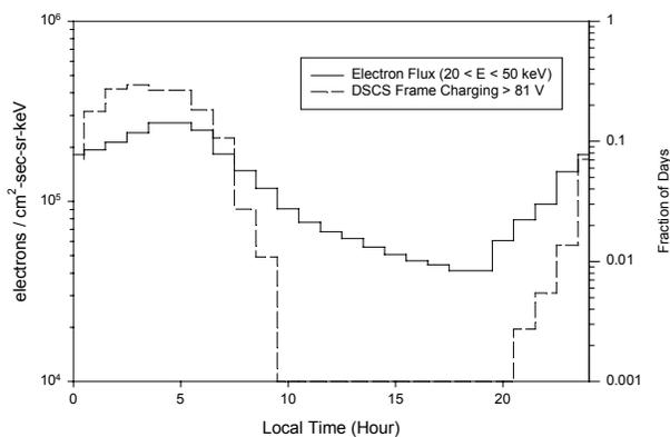
Figure 3. Local time dependence of frame charging and 20-50 keV electron flux as measured by CCS on DSCS.
