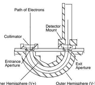
**Figure 3.** A cut-away drawing of a hemispherical electrostatic charged particle analyzer.
