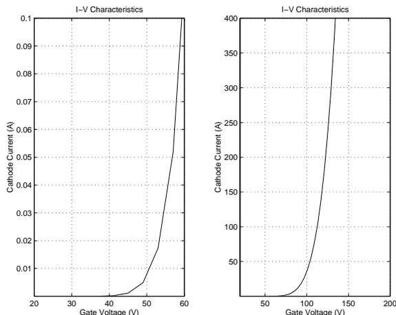
**Figure 3.** Modeled values of emitted current vs. gate voltage for a 5 million tip Spindt cathode array.
