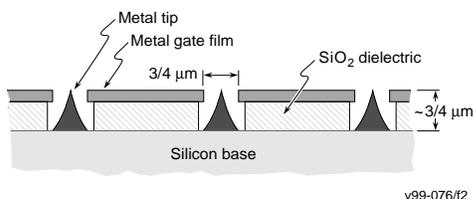
**Figure 2.** Schematic of a Spindt cathode array.
