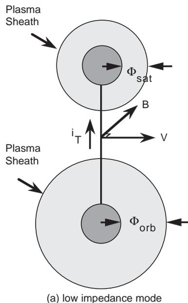
**Figure 4.** Schematic of an electrodynamic tether system flowing current.
