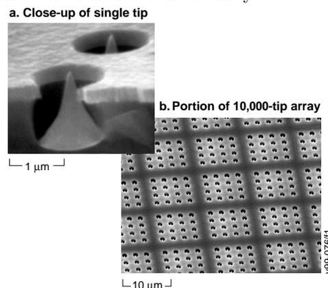
**Figure 1.** (a) Electron micrograph close-up of Spindt cathode tips, and (b) close-up of a section of a cathode array.
