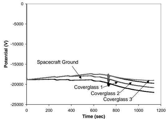
**Figure 3.** Time dependence as computed by NASCAP/GEO.
