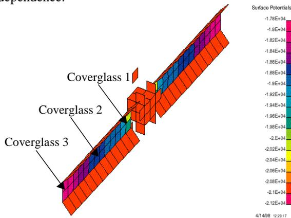
**Figure 2.** Surface potentials as computed by NASCAP/GEO after 1000s.
