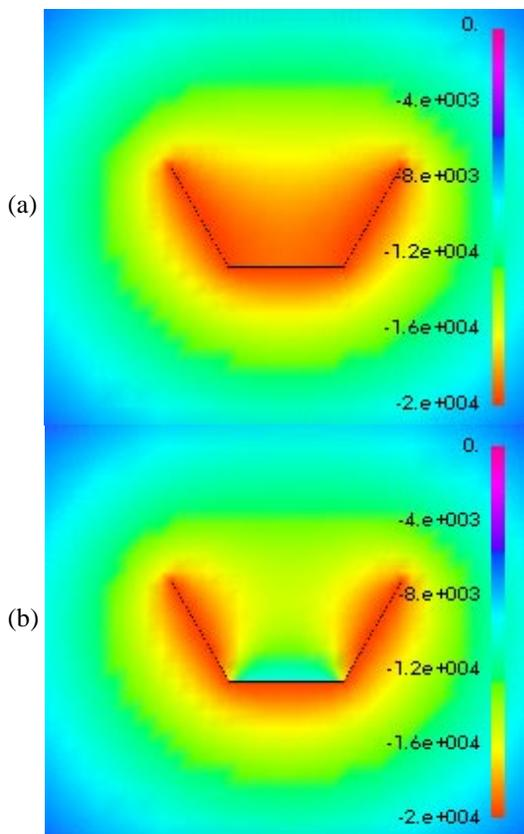
**Figure 4.** Potentials in space about the solar array wing as computed by NASCAP/LEO. The concentrator surfaces and the solar array back are at  $-20$  kV. The coverglass has zero electric field in (a) and is at  $-10$  kV in (b). (a) is physically correct.
