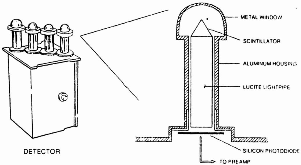
Fig. 1. Diagram of programmatic detector with four input channels. Charged particles enter through metal window and strike scintillator, whose light is seen by photodiode.
