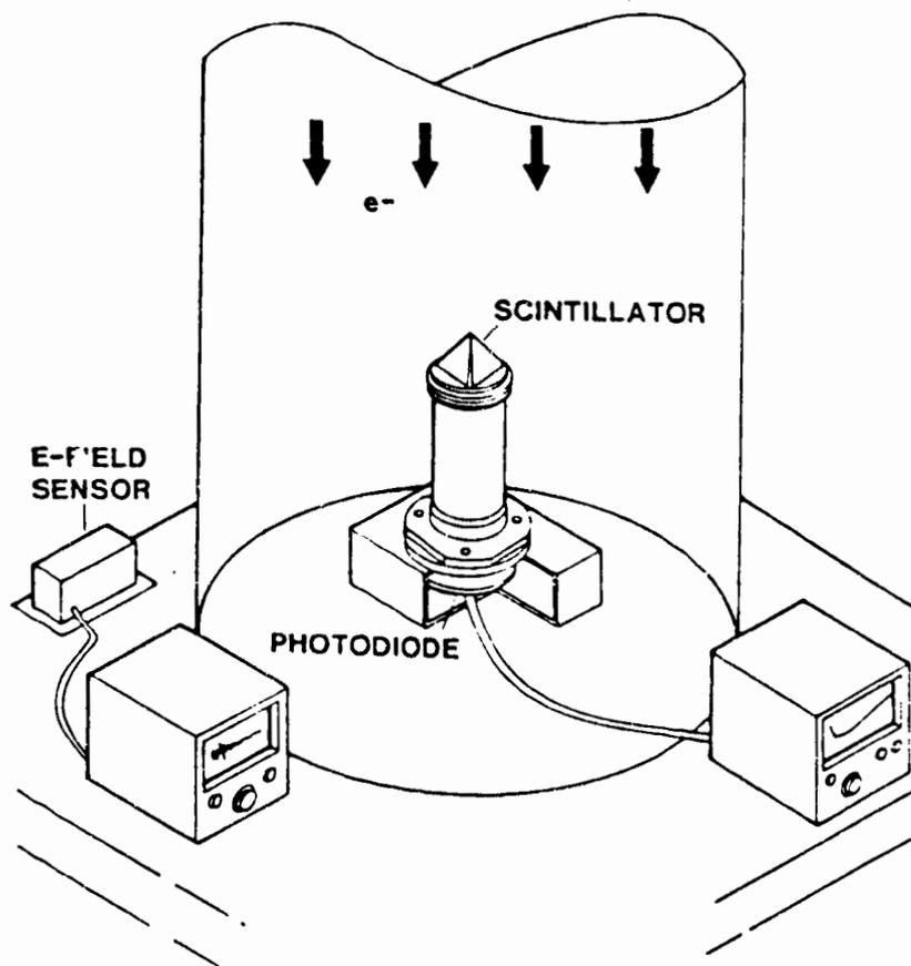
Fig. 7. Diagram of the simulation experiment showing a front end assembly in an evacuated bell-jar, equipped with an electron gun at the top. Light output from the photodiode and the signal from an rf sensor (external to the chamber) were recorded on oscilloscopes.
